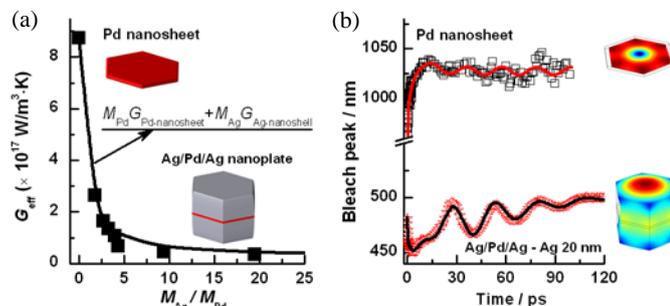
Figure 1. Electron-phonon coupling constants of Pd nanosheet and Ag/Pd/Ag nanoplates (a) and coherent acoustic phonon vibration represented with oscillation of bleach peak wavelength for Pd nanosheet and Ag/Pd/Ag nanoplates with 20 nm Ag shell thickness (b).
