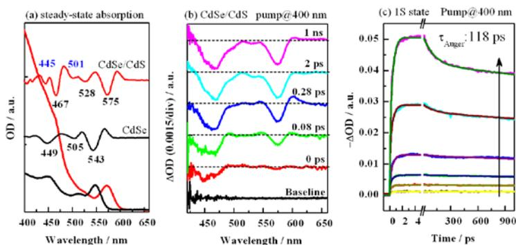
Figure 2. Steady-state absorption spectra and the second derivatives of CdSe core and CdSe/CdS core/shell QDs (a), transient absorption spectra with low shell excitation intensity (b) and Auger recombination lifetime determined from excitation intensity dependence of the decay profiles at the band edge of CdSe/CdS core/shell QDs (c).
