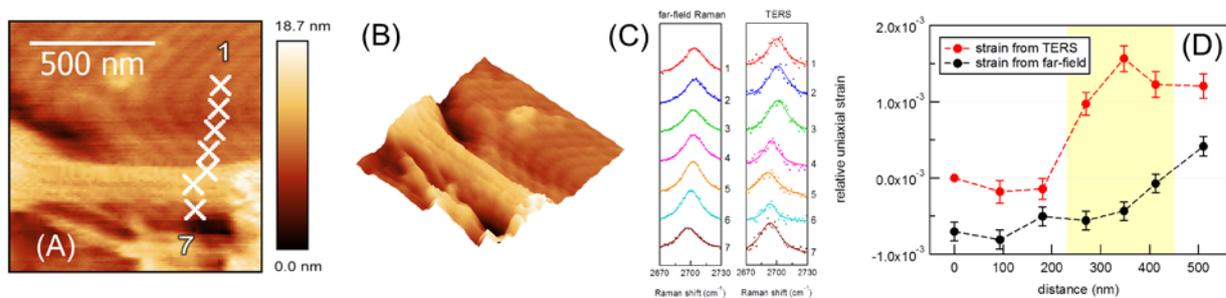
Figure 1. (a) AFM topology of graphene nanoridge. (b) 3D image of (a). (c) G' band in Raman and TERS spectra from each measurement point in (a). (d) graph of strains calculated from band position in (c)
