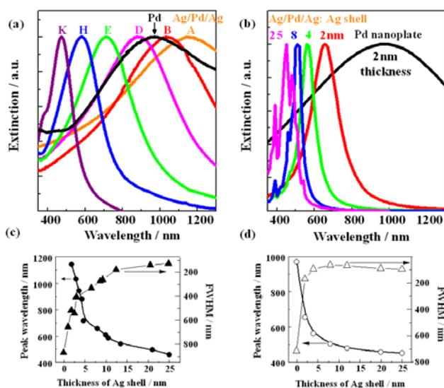
Figure 2. Experimental extinction spectra and the corresponding peak wavelength and full width at half maximum (FWHM) of Pd and Ag/Pd/Ag nanoplates (a and c). Simulation extinction spectra of Pd and Ag/Pd/Ag nanoplates with 2, 4, 8, 12, 20, and 25 nm Ag shell thickness (b and d).
