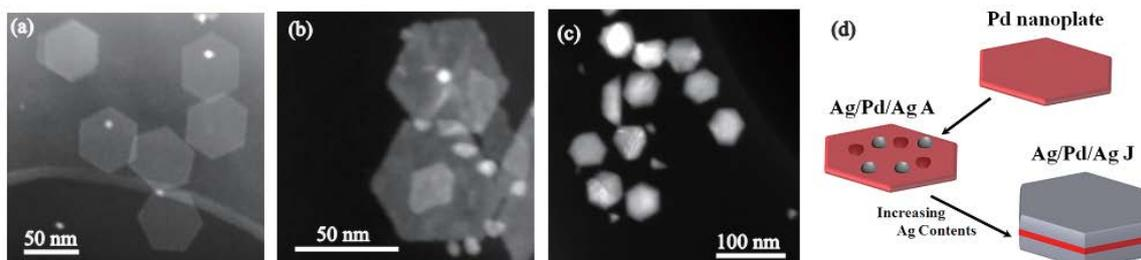
Figure 1. TEM images of Pd nanoplates (a) and Ag/Pd/Ag sandwich nanoplate with two different Ag contents (b and c for the samples labeled with Ag/Pd/Ag A and Ag/Pd/Ag J in the text). Schematics of hexagonal Pd nanoplates, Ag/Pd/Ag A (Ag nanoparticle decorated on both upper and bottom planes of Pd nanoplates), and Ag/Pd/Ag J (thick Ag shell coated on both planes of Pd nanoplates) (d).
