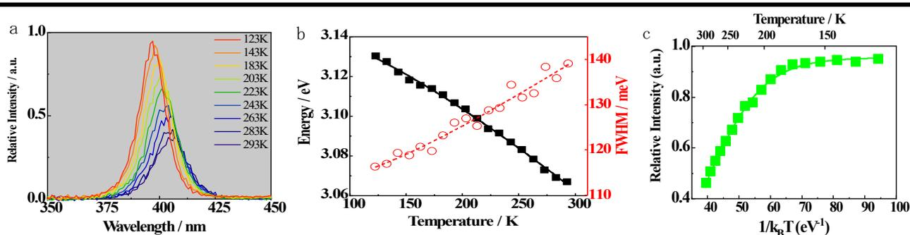
Figure 1. (a) Temperature dependent PL spectra, (b) PL peak energy and FWHM, and (c) PL intensity of ZnSe/ZnS core/shell QDs with PL peak at 406 nm in isopentane.
