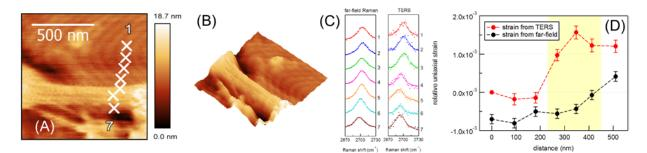
Figure 1. (a) AFM topology of graphene nanoridge. (b) 3D image of (a). (c) G' band in Raman and TERS spectra from each measurement point in (a). (d) graph of strains calculated from band position in (c)
