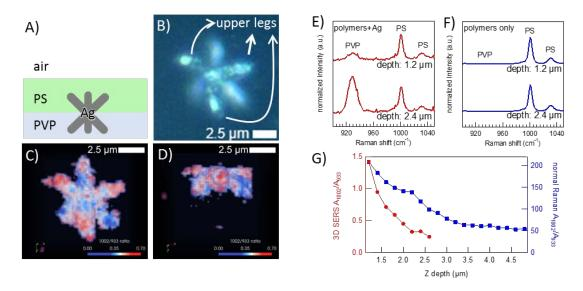
Figure 2. A) A SERS spectrum of PATP from the center of a hexapod silver microstructure. B) Optical microscope image of the particle. C),D) Top and diagonal views 3D SERS images constructed by PATP a1 mode at 1074 cm-1, using the same particle as B). E) Examples of 2D slices in the Z axis of B). Only one in five slices (corresponding to  $1.5 \mu m$  distance) are shown. Noted that C), D) and E) use the same color scale.
